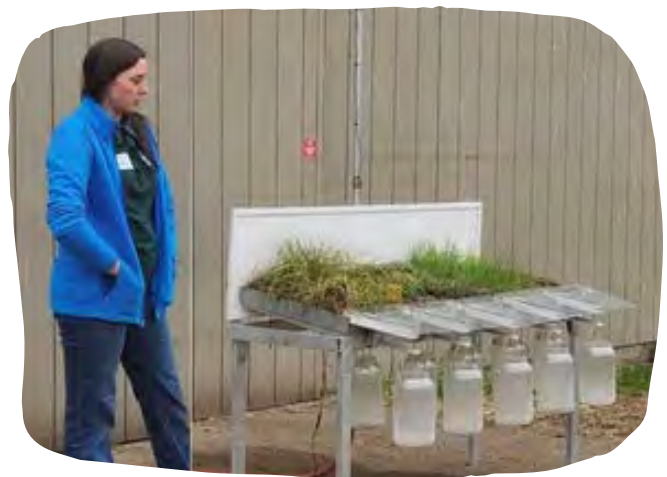
Theresa Brehm of Natural Resources Conservation Service uses a rainfall simulator to discuss managing land for soil health.
